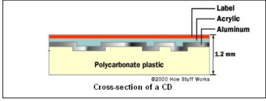
it if you scratch it or even write on the label with a ball-point pen. Even some felt-tipped pens can be dangerous, because the solvent used in the ink can dissolve the acrylic and destroy the bumps, too. Sharpie brand markers are generally pretty safe because their solvent evaporates relatively quickly.
