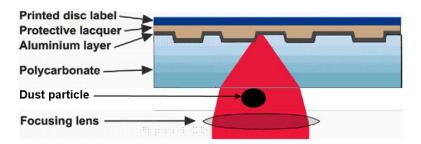
of the disk, and that bending focuses the beam to a tiny spot right where the metal layer with the bumps is. This means that little scratches or dust particles won't block the whole beam, and the laser can read right through them!
